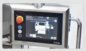
Control by 10" industrial PC touch screen: screen integrated features (production data, test screen, machine manuals, videos, driver download...).
